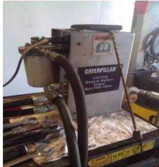
200 gallon day-tank used to supply ULSD#2 for test. Close-up of AIC-6008 fuel flow meter
