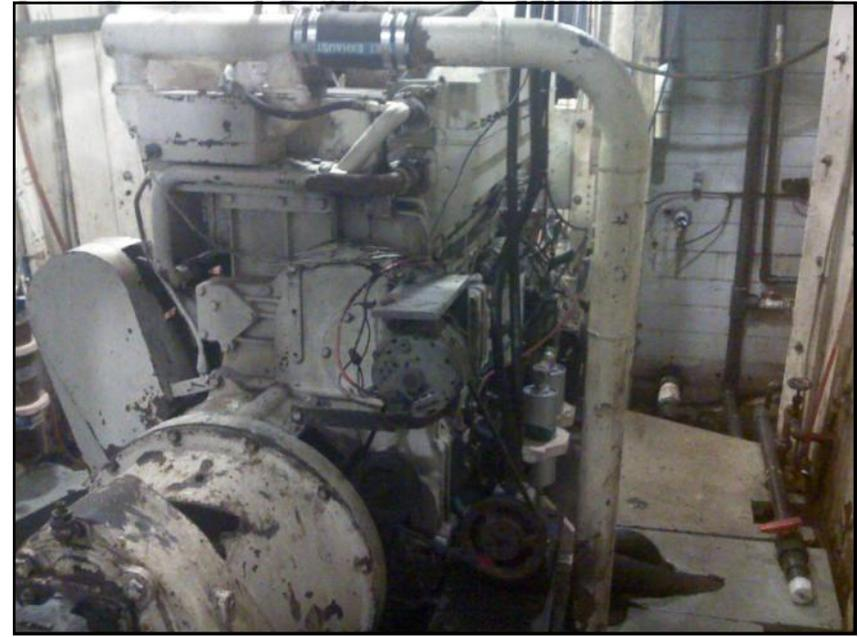
Cummins KTA1150 main propulsion engine with dual Fitch Heavy-Duty units mounted in series on RHS of engine using wooden support bracket. Close up of installation shown below. Fuel flows from filters on right through both Fitch units into injector pump on left.
