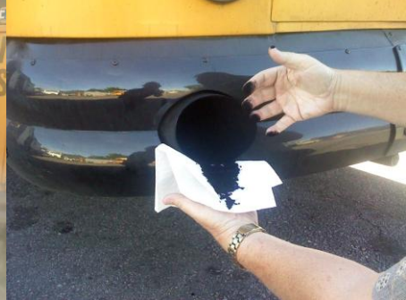
Accumulated soot in tailpipe
